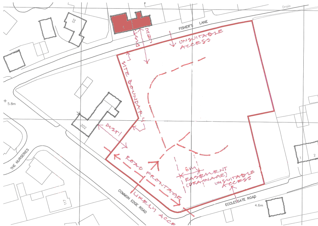
Constraints plan (taken from the Design & Access Statement) shows the listed cottages in red.
